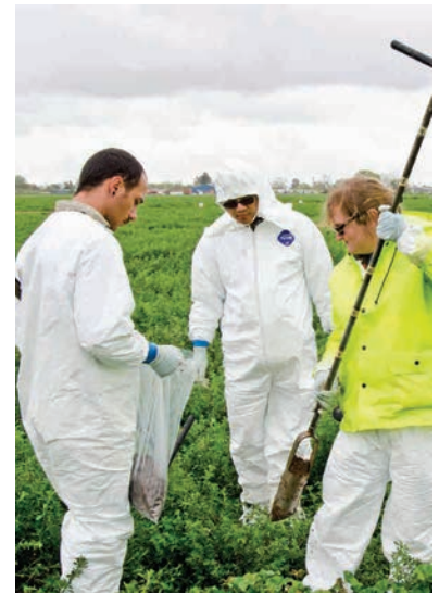
DPR scientists take soil core samples in an alfalfa field at the University of California, Davis, to determine various soil properties.
