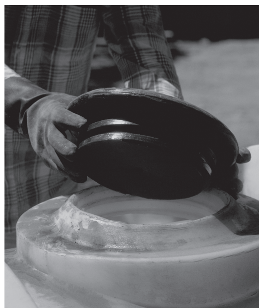
FIGURE 5-8: Employers must equip all openings on tanks used for mixing or applying pesticides with tightly-fitting covers that prevent splashes or spills.
