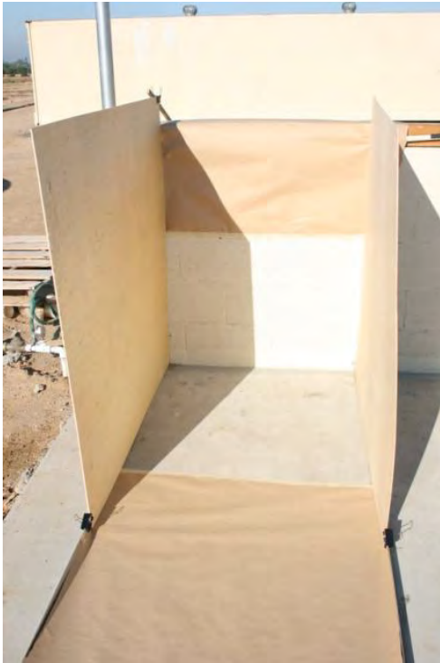
Figure 3. Masking an area to be treated. This example was 2-ft up and 3 ft out.
