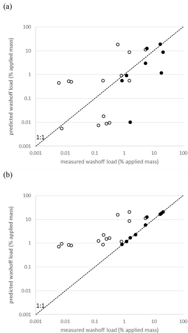
Figure 3. PRZM-predicted pesticide washoff loads from impervious surfaces relative to measurements (3, 4, 16, 20), (a) with repeated soil  $K_d$  (partitioning coefficient), and (b) with  $K_d$  calibrated to measurements at 1DAA (days after application). Open circles for data at 1DAA (days after application) and closed circles for those >1DAA
