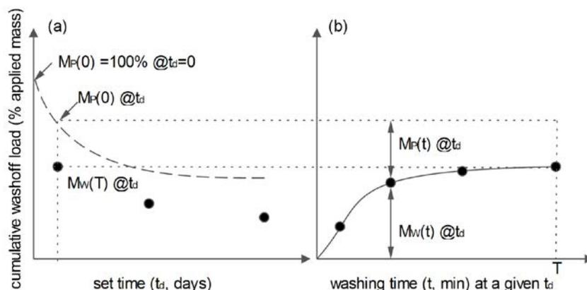
Figure 1. (a) Washoff potential,  $M_p(0)$  (dashed line) and total washoff load,  $M_w(T)$  (dots) are presented at a given set time  $t_d$ . (b) Cumulative washoff loads,  $M_w(t)$  (dots) and washoff profile (solid line) measured during washing time  $t$  ( $t=0\sim T$ ). Note: Dotted lines included to connect  $M_p(0)$  and  $M_w(T)$  in the two panels.
