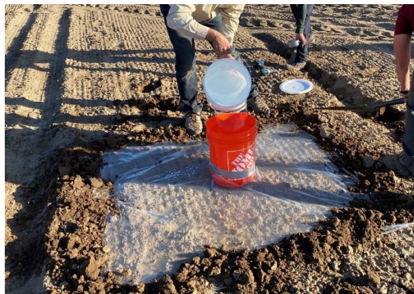
Figure 4. Covering the edge of the plastic sheet/tarp with soil and filling the bucket with water.
