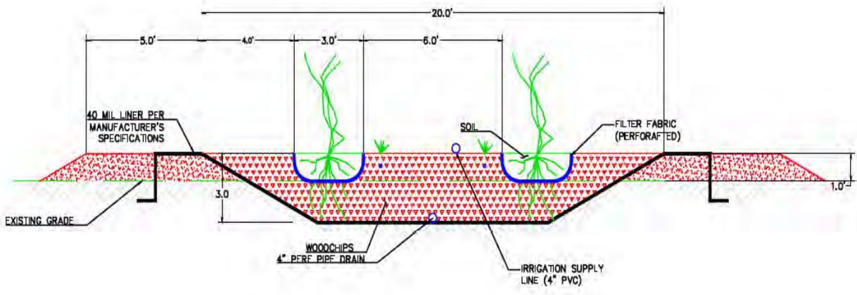
Figure 4. Cross section of bioreactor.
