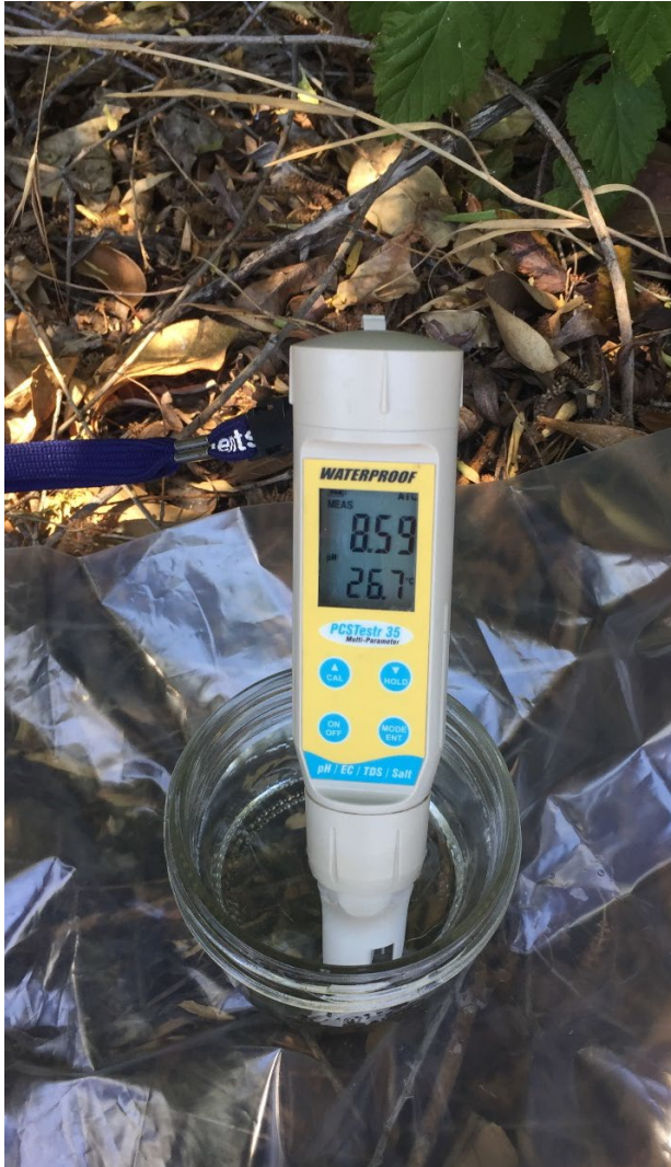
Figure 3. pH meter submerged in half-pint glass jar filled with a water sample.
