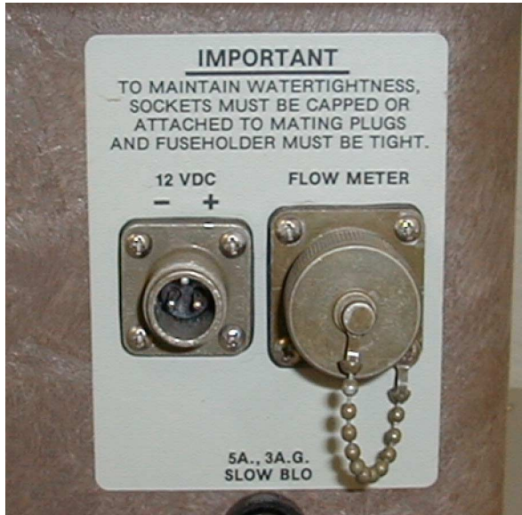
Figure 4: Connectors for battery and liquid level actuator on models 2700 and 2700R
