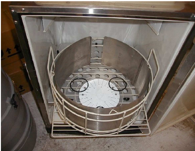
Figure 6: Bottle rack and retaining ring, inside refrigerator compartment, for model 2700R
