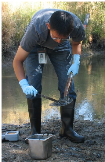
Figure 4: Collecting a grab sediment sample into a stainless steel container
