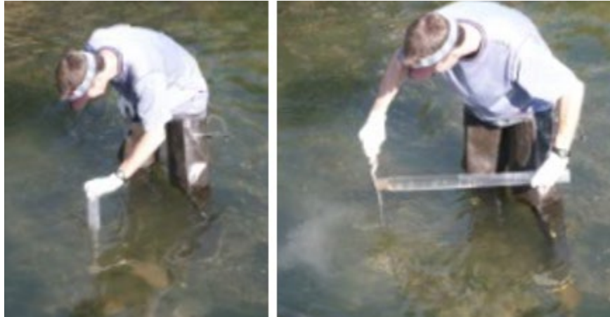
Figure 6: Sediment collected with polycarbonate tube
