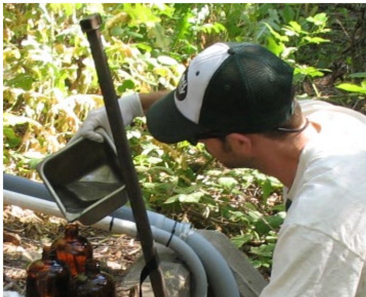
Figure 2: A stainless steel secondary container used in sampling shallow waters
