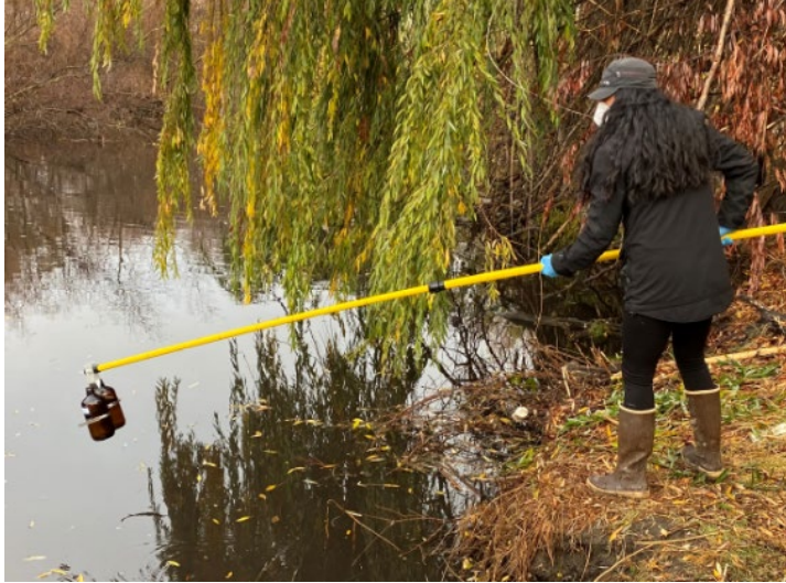
Figure 1: A sampling pole used in grab sampling
