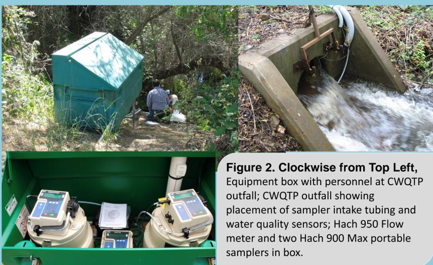
Figure 2. Clockwise from Top Left, Equipment box with personnel at CWQTP outfall; CWQTP outfall showing placement of sampler intake tubing and water quality sensors; Hach 950 Flow meter and two Hach 900 Max portable samplers in box.
