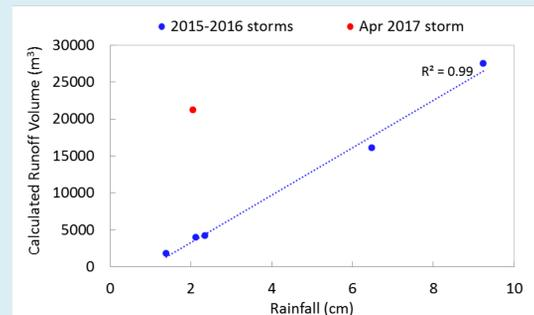
Figure 4. Correlation between rainfall and calculated water volume through the CWQTP. Red marker (April 2017 storm) not included in correlation.
