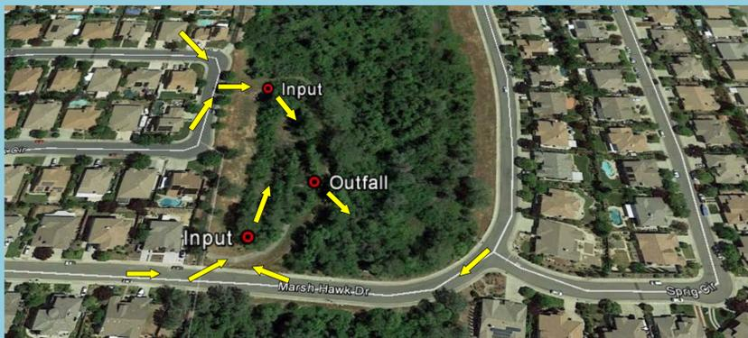
Figure 1. CWQTP in Folsom with flow schematic (Google Earth image)
