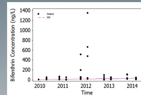
Figure 6. Trend in bifenthrin concentrations at stormdrain outfalls in southern California. Samples were collected during rainstorm sampling (p=0.008)
