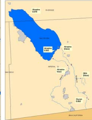
Figure 3. Herbicides detected (concentrations in \mu\text{g L}^{-1} or trace detections) in Imperial County. Water samples taken where no herbicides were detected are marked with the symbol (•).
