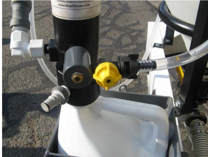
Photo One: GTP pumping component attached to container
