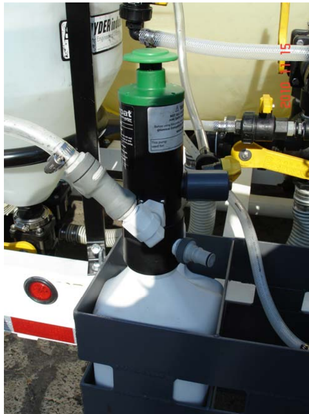
Photo Two: GTP pumping component attached to container, showing dry couplers
