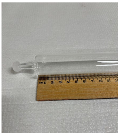
Figure 17: The proper placement of the ruler when measuring the placement of fill lines to be drawn.
