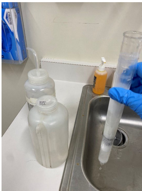
Figure 9: Flushing of the combustion tube after saltwater TOC analysis. Turn off furnace and ensure the combustion tube has cooled prior to flushing.
