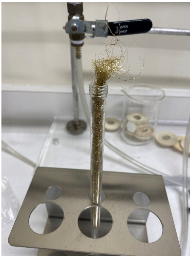
Figure 20: Packing fresh brass wool into the absorption tube.
