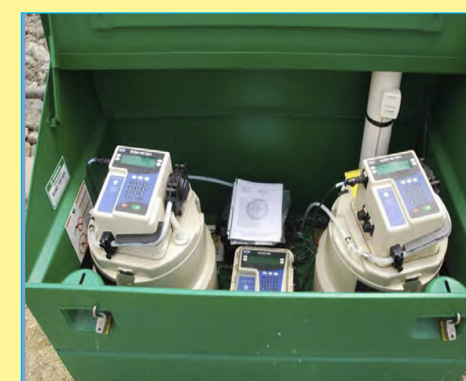
Two Hach Sigma 900 MAX automated samplers with a Hach Sigma 950 (center). (L.R. Oki)
