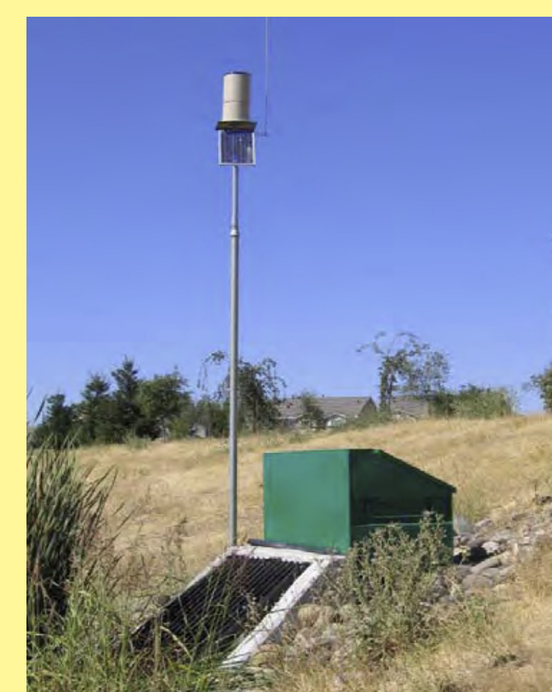
Site NAT (Sacramento County), the green box holds the data logger and automated sampler, the rain gauge is to the left. (L.R. Oki)
