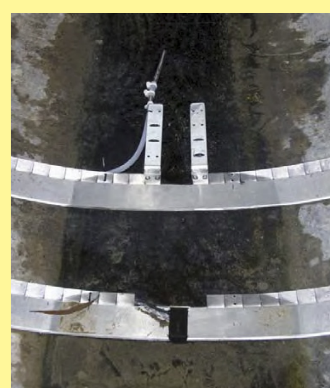
Electrical conductivity and pH sensor (top band) and velocity sensor (bottom band). The intake tube for the automated sampler is attached on the top left sensor cover. (L.R. Oki)
